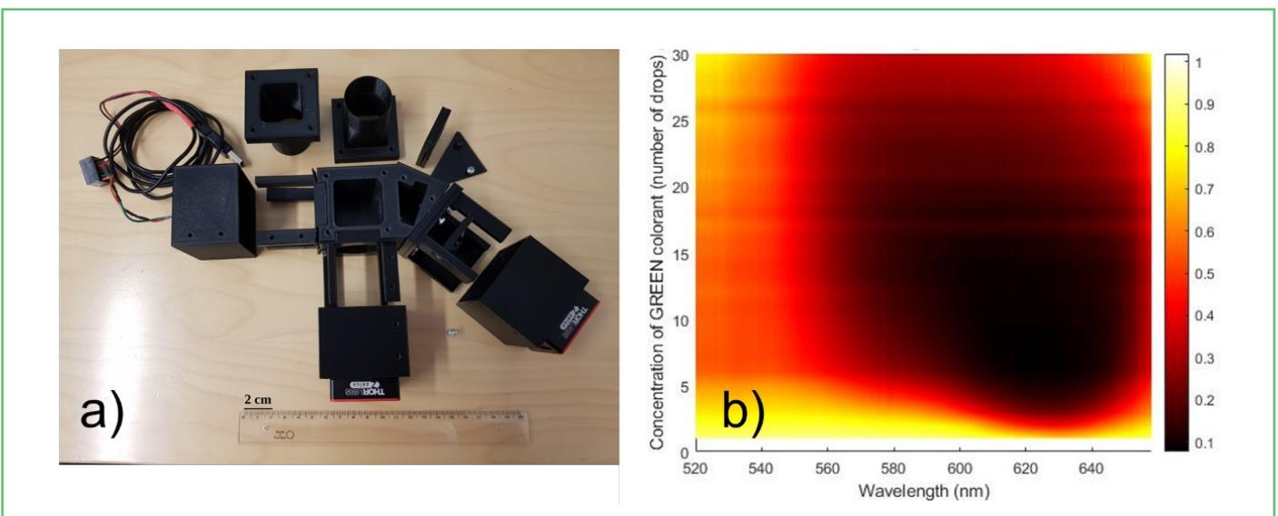
Figure 19: a) Unassembled prototype including all the parts for imaging and spectroscopic measurements. b) example of results, i.e., a map showing the spectra as a function of red-dye concentration in water.
