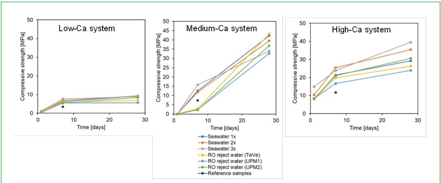
Figure 13: Compressive strength of binders prepared with different high salinity waters using metakaolin (low-Ca system), mixture of metakaolin and blast furnace slag (medium-Ca system), and blast furnace slag (high-Ca system). Seawater 1x, 2x, and 3x refer synthetic seawater with 1x, 2x, or 3x salt content.
