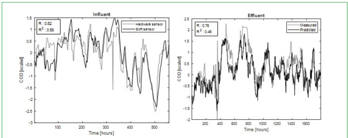
Figure 6: The independent 23-day testing period of the developed soft sensor for influent COD and the independent 75-day testing period of the predictive model for effluent COD.
