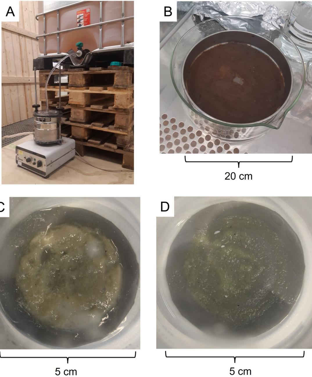
Figure 18: A) Filtration of 1 m<sup>3</sup> of P&P effluent, B) the untreated sample representing solids (>20 μm) from 1 m<sup>3</sup> of P&P effluent, C) the solids (>20 μm) from 250 L of P&P effluent after one H<sub>2</sub>O<sub>2</sub> treatment, and D) the solids (>20 μm) from 250 L of P&P effluent after two rounds of NaOH-Urea treatment in combination with H<sub>2</sub>O<sub>2</sub> treatment.
