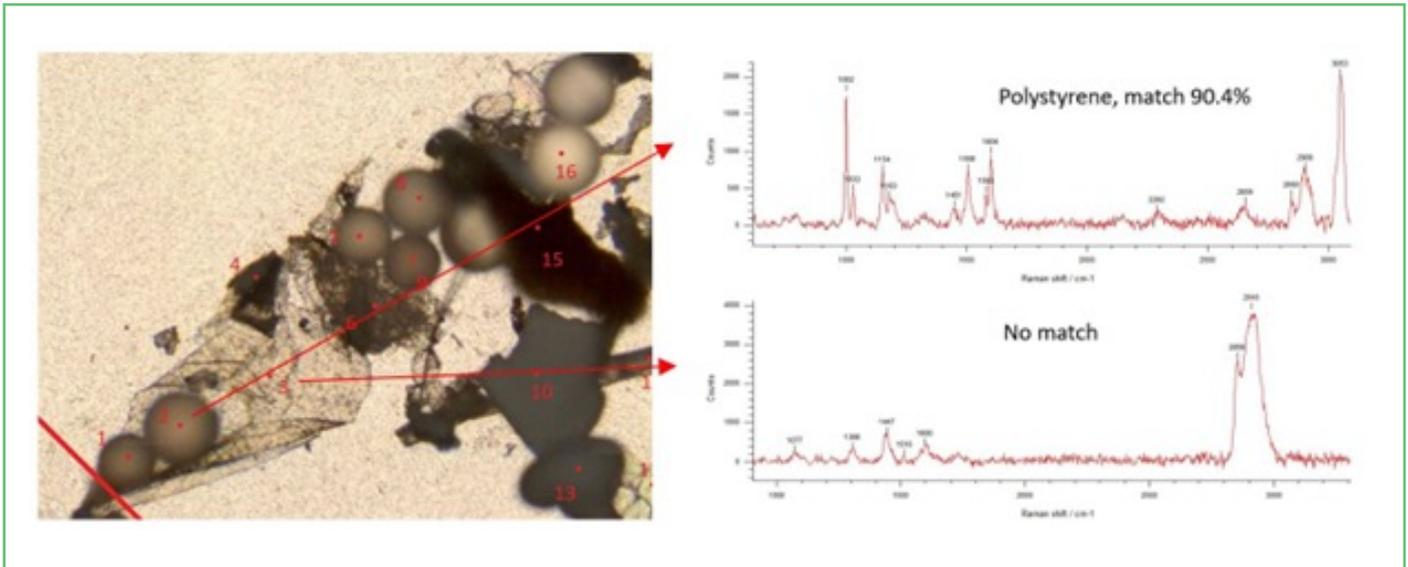
Figure 21: Left: Particles extracted from sewage sludge for Raman analysis on a filter. Right: Examples of Raman spectra of the analysed particles.
