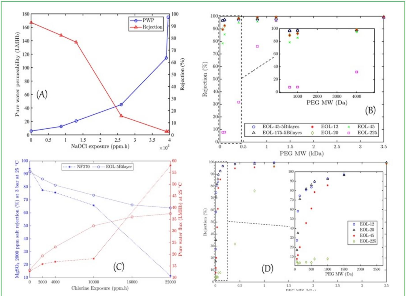
Figure 14: The effect of NaOCl exposure on: PWP and salt rejection (A); Retention of PEGs and PWP of oxidised and LBL-coated membranes (B&D); Stability of 5 bilayer coated and commercial membrane NF270. (The Numbers denoted to the name of EOL membranes are the permeability of membranes).
