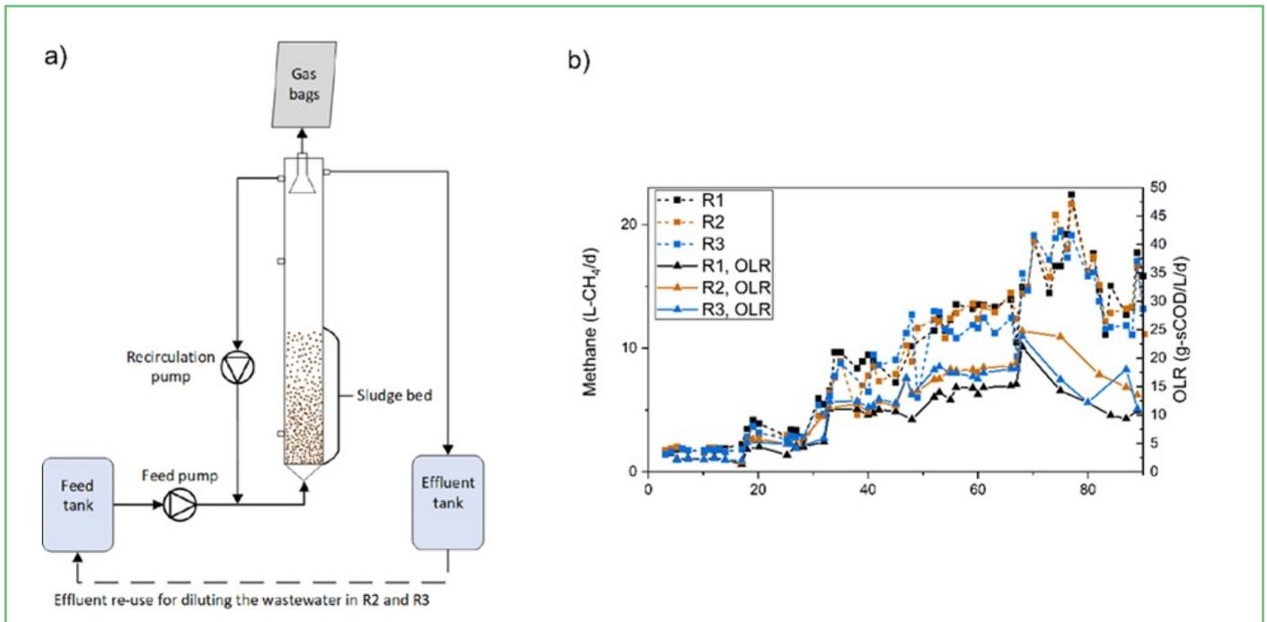
Figure 12: Process scheme (a) and methane production at different OLRs (b).
