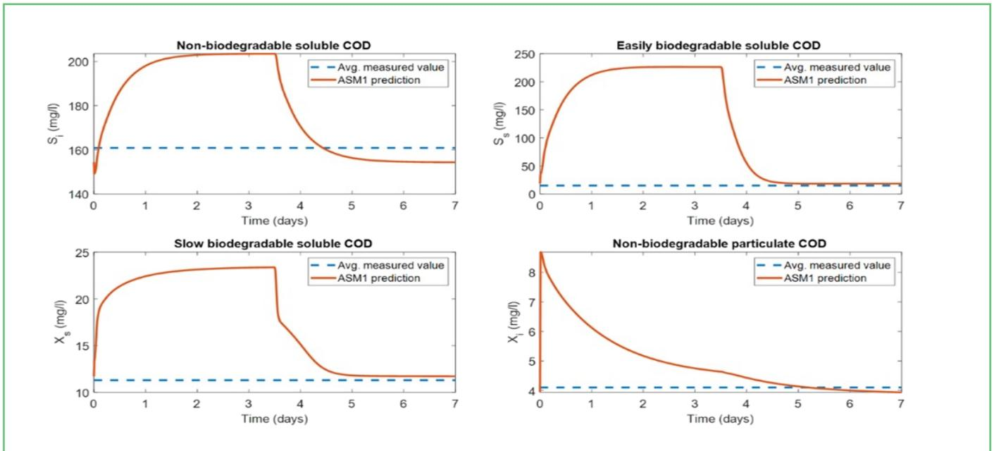
Figure 7: Calibration of the ASM1 model using collected COD samples.
