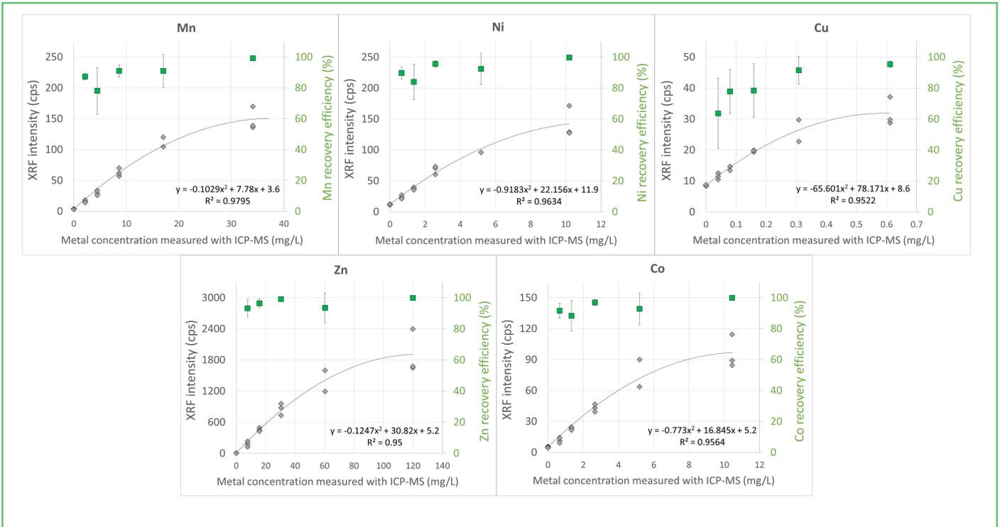
Figure 10: The metals were precipitated in-situ on/in the metal collecting filter and analysed directly from the filter with a portable XRF device. X-axis is the real metal concentration obtained with inductively coupled plasma mass spectrometry (ICP-MS) and the Y-axis is the fluorescence intensity measured with XRF. The data is used for the site-specific calibration of the system.
