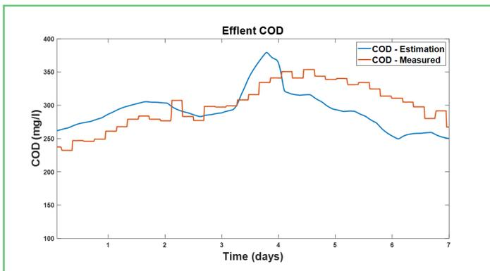
Figure 8: Comparison of the estimated effluent COD generated by the ASM1 model with the effluent COD measurements obtained through the online monitoring system in the WWTP.
