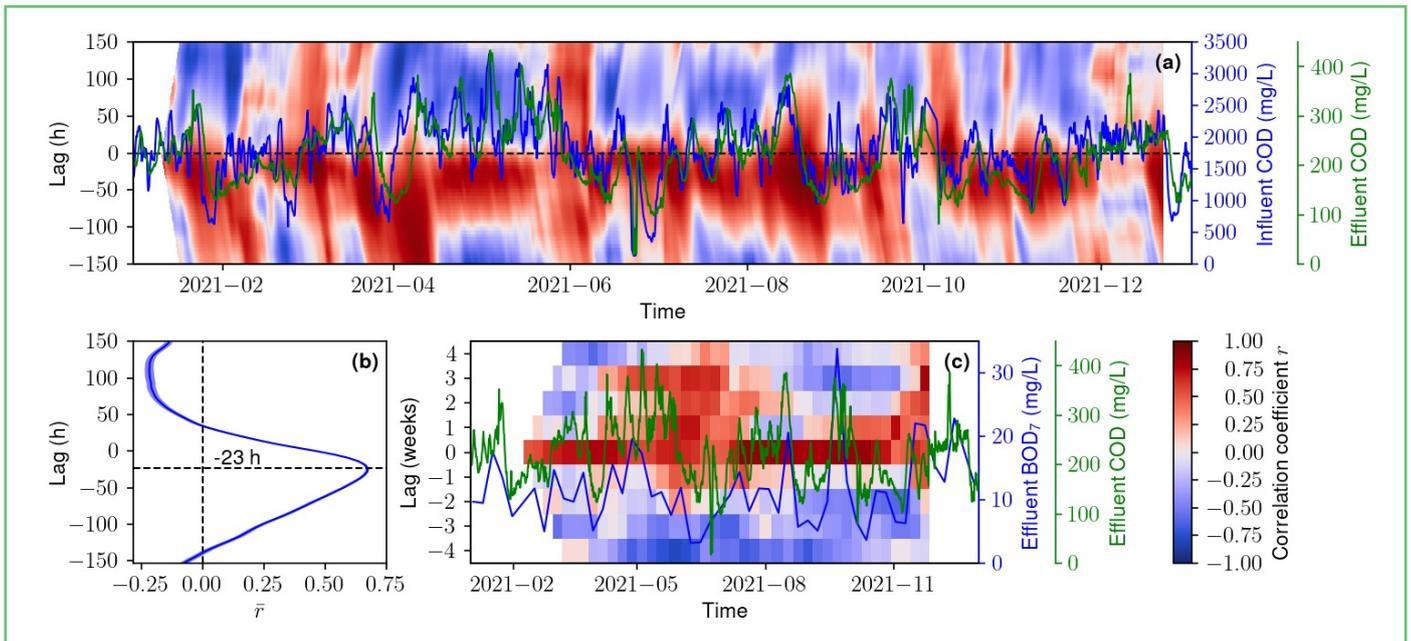
Figure 9. (a) Time-dependent cross correlation (colour map) between the influent and effluent COD for different lags. (b) Average cross correlation for each lag. (c) As in (a) but for effluent COD and BOD.
