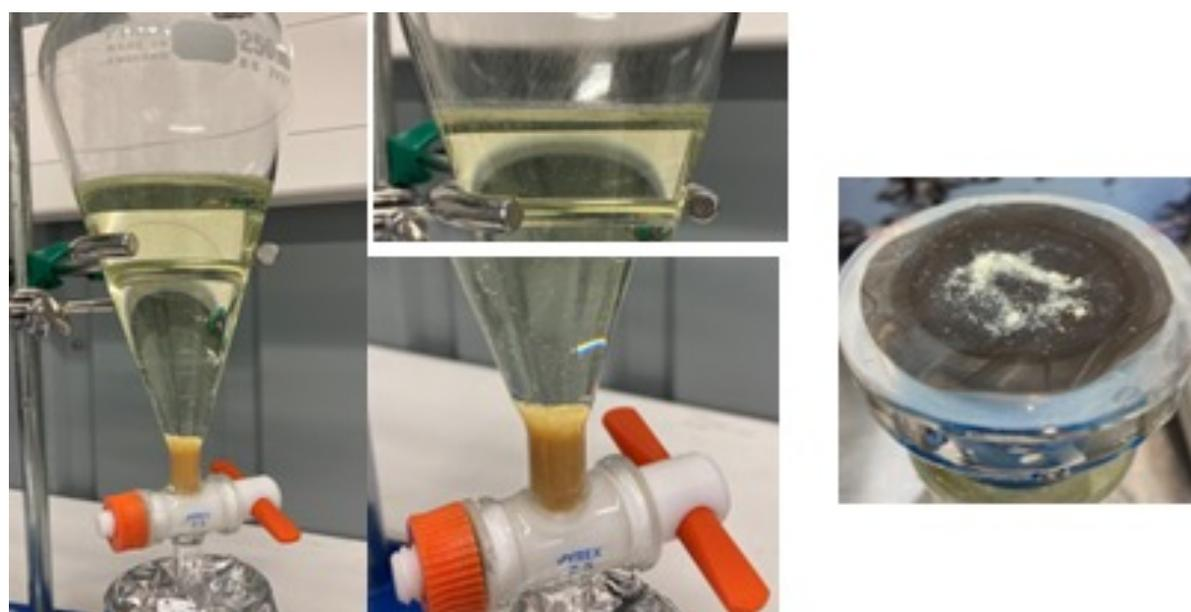
*Figure 17: MP separation process optimisation of the fibrous sludge. Despite the successful density separation step, the process still required optimization of the chemical-enzymatic phase to reduce the amount of remaining solids to be analysed with spectroscopy.*
