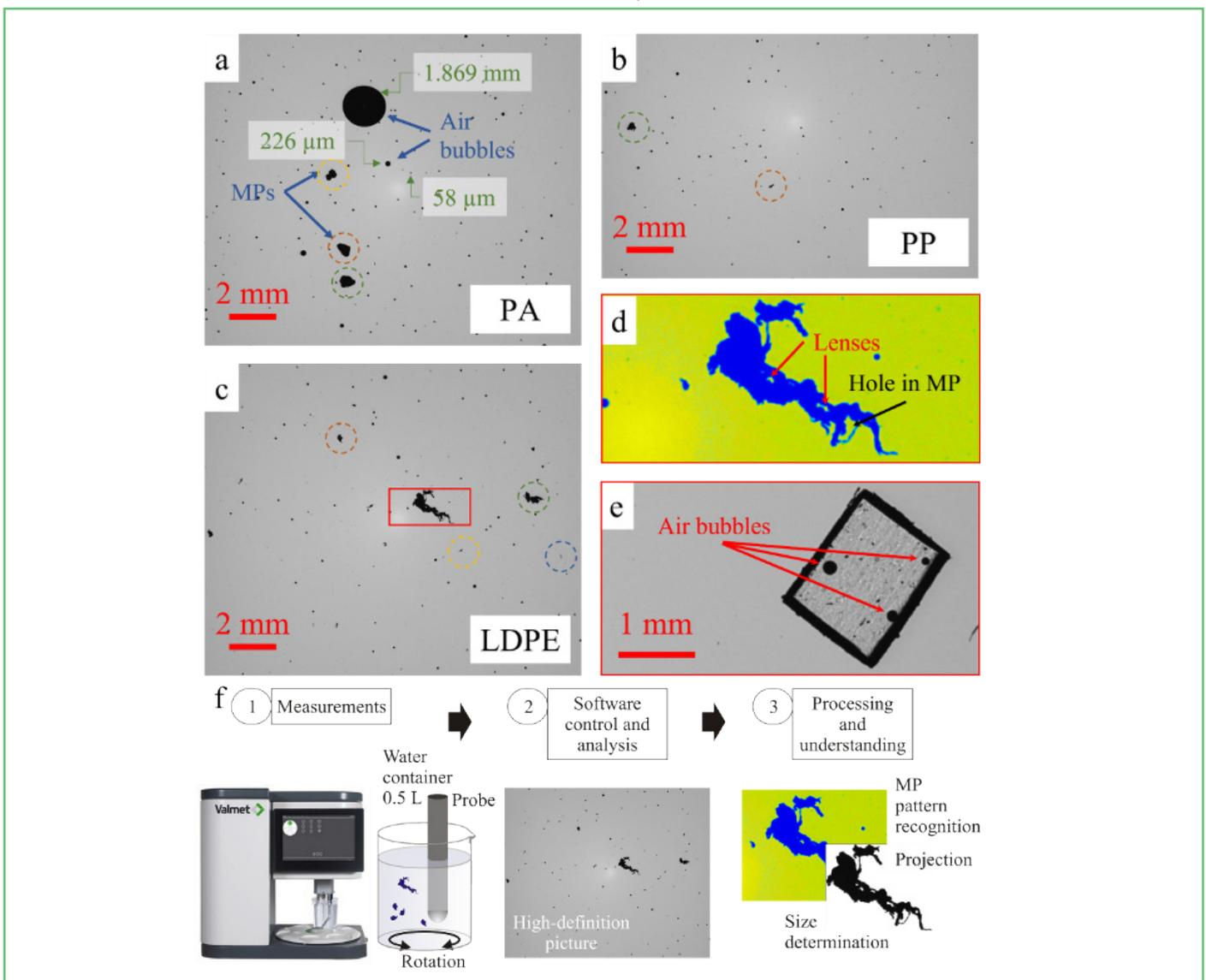
Figure 20: Images acquired with the Valmet FS5 UHD device for different samples in water including a) PA particles, b) PP particles, and c) LDPE particles. d) zoomed-in and enhanced image of a microplastic particle from c) (red contour). Red arrows in d) highlight bright “lensing” areas in the microplastic particle. Black arrows in d) highlights a hole in the MP. e) air bubbles on a PET MP. f) Procedure to image and recognise MPs in a water sample [Pub1].
